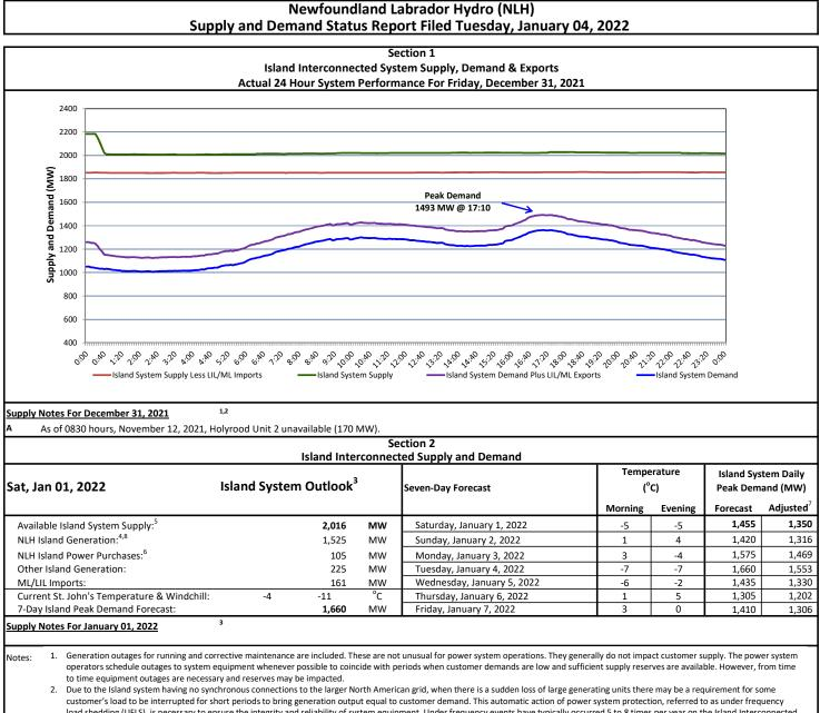
load shedding (UFLS), is necessary to ensure the integrity and reliability of system equipment. Under frequency events have typically occurred 5 to 8 times per year on the Island Interconnected System and the resultant customer load interruptions are generally less than 30 minutes. With the activation of the Maritime Link frequency controller during the winter of 2018, UFLS events have occurred less frequently.
